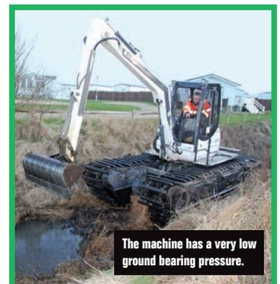
The machine has a very low ground bearing pressure.
