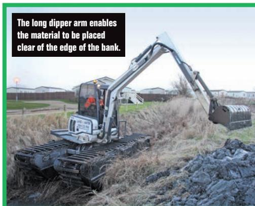
The long dipper arm enables the material to be placed clear of the edge of the bank.
