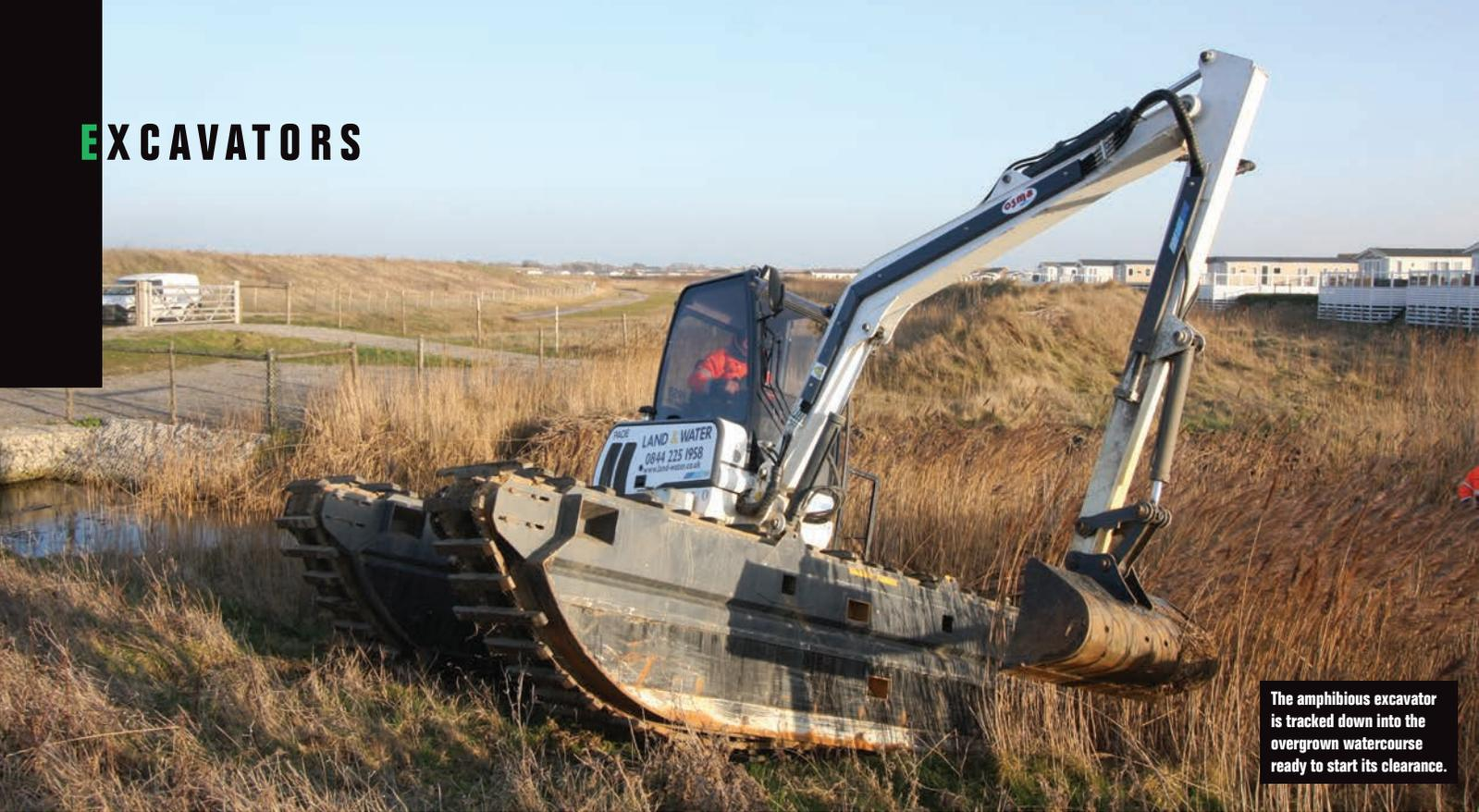
The amphibious excavator is tracked down into the overgrown watercourse ready to start its clearance.
